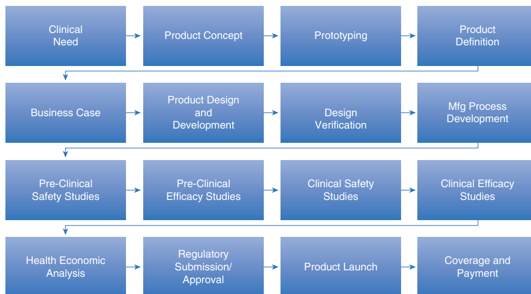
FIGURE 1 Illustration of the product development process. Any successful product development effort must navigate most, if not all, of the steps defined in this sequence. Depending on the device, drug, biologic, or combination designation, plus the Class of the product (I, II, or III), the requirements for Clinical Studies will vary from none to multiple randomized controlled clinical trials. The precise sequence of these steps may also vary depending on the nature of the product.
